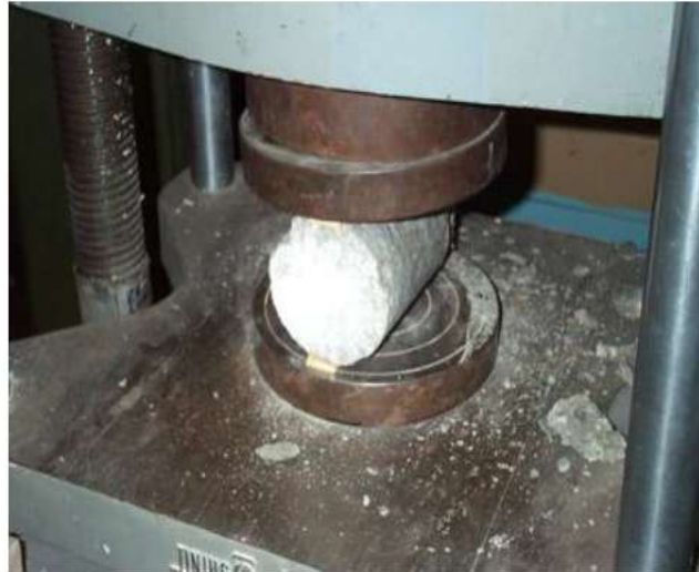
Fig 5: Testing of split tensile
